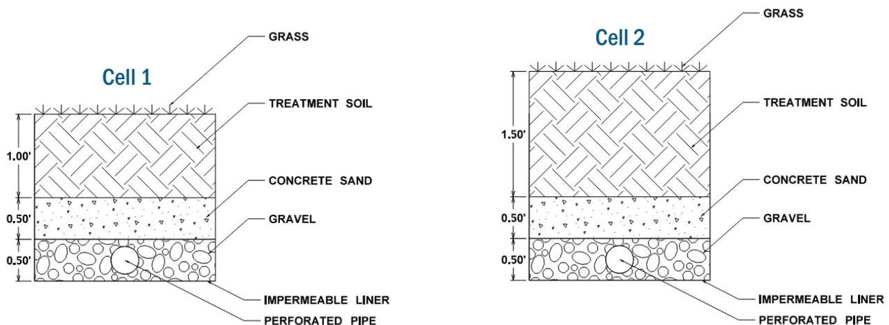
Figure 1. Cross Section of the Bioretention Cells: 12-inch BSM (cell 1) and 18-inch BSM (cell 2)
